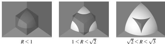
Figure 8: Three cases for the intersection of eighth ball and unit cube.
